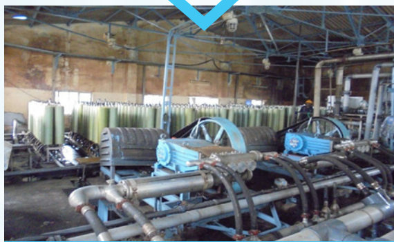
High Pressure Reverse Osmosis Plant at Nira
